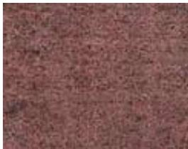
**Synthetic fibers / synthetic felt** include nylon, polyester, polypropylene, and acrylics, which are needle-punched into relatively dense cushions which have a firm feel and, as with other types of cushion, can be made in virtually any weight, to stand up under light, medium, or heavy traffic, which is how they are usually classified.
