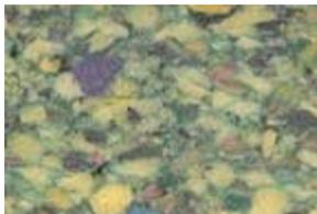
Rebond pad usually contains BHT (Butylated Hydroxytoluene). BHT is a common preservative used in many plastics and even in bread. BHT was removed from most olefin backings in 1985 because of yellowing of carpet fibers. Many cushion manufacturers have now also removed BHT from their products.
