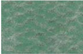
**Flat sponge rubber** is a firm, dense cushion, which has a flat surface and is normally used in large-scale commercial applications and with loop type (or berber) carpet.
