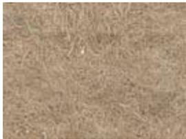
**Natural fibers** include **felt**, **horsehair**, and **jute**. These are, of course, highly susceptible to rotting if over-wetted, odor development, and natural degradation. Some natural fiber cushions have been treated with a water-soluble dye that can stain a wet carpet. Fiber pads are used sometimes to limit the movement in an area rug. The key is density. Felt cushion density is by weight of ounces per square yard.
