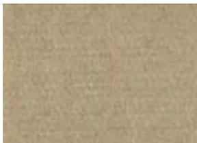
**Mechanically frothed urethane foam** is made with carpet backing machinery. Frothed urethane cushions are made from a process originally developed to apply cushioned backings to carpet. The urethane foam cushioning is applied to a sheet of nonwoven material, forming a carpet cushion product with a typically higher density and firmer feel.
