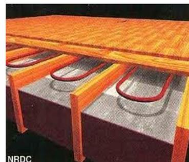
**When installing flooring over Radiant Heat, the heat is to be encased into the subfloor or covered with a cementitious patching compound. The Radiant Heat should not come into direct contact with the flooring.**
